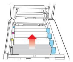
**6.** Put the cartridge down gently onto a piece of paper to prevent toner from marking your furniture and to avoid damaging the green drum surface.
